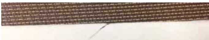
Fiberglass fabric with Fraying
